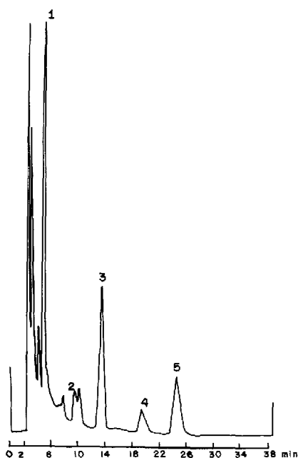
Fig. 1. Separation of an artificial mixture of five principal opium alkaloids. Column: \mu Bondapak phenyl (300 mm \times 3.9 mm I.D.). Eluent: water (1%, w/v sodium acetate and 7.0 mM triethylamine-methanol (42:58). Flow-rate: 1.0 ml/min. UV detection at 254 nm. Peaks: 1 = morphine; 2 = codeine; 3 = papaverine; 4 = thebaine; 5 = noscapine.
